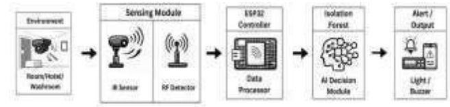
Fig. 1. System Architecture of the Proposed Smart Anti-Spy Camera Detection System
